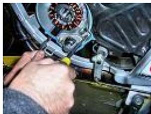
**REMOVE THE TWO SCREWS OF THE PICK UP, WITH A CROSS-SHAPED SCREWDRIVER.**
