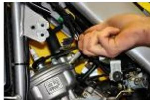
**IF YOU DON'T HAVE A COMPRESSED AIR GUN, REMOVE THE SPARK PLUG, WITH A KEY OF 21.**
