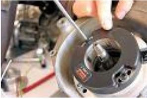
**RECOVER THE WIRE PASS OF THE ORIGINAL STATOR AND PLACE IT IN THE RIGHT WAY ON THE TUBE OF PREMIUM STATOR. PLACE THE PREMIUM STATOR ON THE SUPPORT, PUTTING THROUGH THE CARTER HOLE AND TIGHTEN IT, WITH THE 2 PROVIDED SCREWS OF 5X30 MM.**
