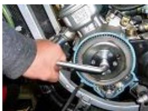
**LOOSEN THE NUT, WITH AN ALLEN KEY OF 15.**
