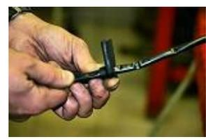
**AFTER RECOVERING THE SHUTTER ON THE TUBE OF THE ORIGINAL STATOR, PLACE IN THE RIGHT WAY, ON THE TUBE OF PREMIUM STATOR.**
