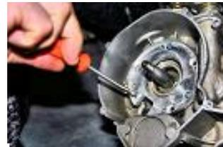
**PUT THE PREMIUM SUPPORT END TIGHTEN IT, WITH THE 3 PROVIDED SCREWS AND A CROSS-SHAPED SCREWDRIVER.**
