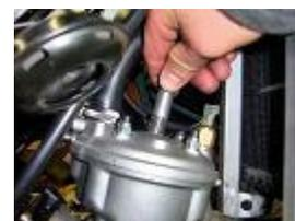
**PUT AT THE SPARK PLUG PLACE, A BLOCK PISTON STICK AND TURN BY HAND THE ROTOR TO PUT THE PISTON IN TOUCH WITH ITS BLOCK PISTON STICK.**
