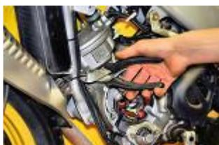
**CUT THE INFERIOR PLASTIC COLLAR OF THE TUBE, UNTIL THE CONNECTOR.**
