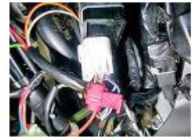
**PLACE THE RED PROVIDED CLIP ON THE BROWN OR RED/WHITE CABLE (FOR THE MODELS MADE SINCE 2008) OF THE ORIGINAL CDI, WITHOUT DISCONNECTING, NEITHER CUTTING IT, PLACE THE BROWN CABLE OF THE DIAGRAM, IN PARALLEL ON THE CLIP NEXT TO THE BROWN CABLE OF THE CDI AND CLOSE THE CLIP WITH PLIERS IN ORDER TO PUT THE 2 CABLES IN TOUCH.**
