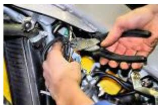
**CUT THE INFERIOR PLASTIC BRIDLE, UNTIL THE COIL.**
