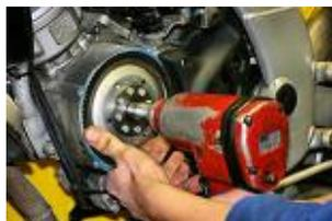
**LOOSEN THE ROTOR NUT OF 15, WITH A COMPRESSED AIR GUN.**
