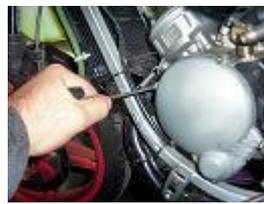
**REASSEMBLE THE IGNITION COVER, WITH AN ALLEN KEY OF 4. PLACE BETWEEN THE IGNITION CARTER AND THE ENGINE, STRUTS TO PULL THE CARTER AND LET THE AIR GO FREELY, OR MADE HOLES IN THE TOP AND THE BOTTOM OF THE IGNITION, TO VENTILATE IT.**
