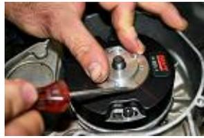
**LOOSEN THE BLOCK PISTON STICK, USE IT LIKE A STICK, TURNING THE CRANKSHAFT TO FIND THE BTDC. AT THE BTDC, MAKE MEET THE RED MARK OF STATOR AND ROTOR. TIGHTEN THE ROTOR WITH THE DISC AND THE ORIGINAL NUT.**
