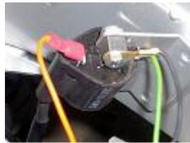
**REMOVE THE ORANGE CABLE FROM THE COIL, TO REMPLACE IT BY THE ORANGE CABLE OF THE DIAGRAM. REMOVE THE SUPPORT SCREW, FROM THE HIGH VOLTAGE COIL, AND FIT, KEEPING THE ORIGINAL BLACK CABLE, AND THE BLACK OF THE DIAGRAM AND THE GREEN/YELLOW OF THE STATOR.**
