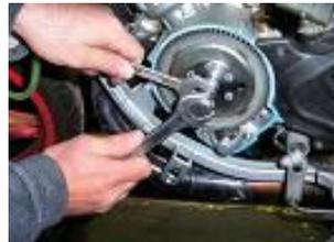
**SCREW THE EXTRACTOR FOR YAMAHA IGNITION AND REMOVE THE ROTOR, WITH THE 2 KEYS.**
