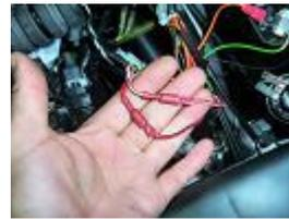
**CONNECT THE RED/BLACK CABLE OF THE DIAGRAM AND THE STATOR TOGETHER.**
