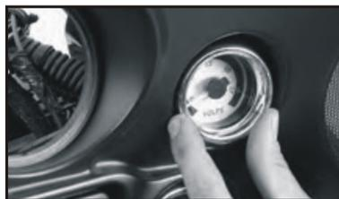
6. Remove the meter from the inner fairing.
