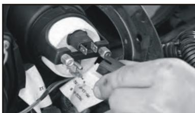
4. Disconnect the wiring from the speedometer, tachometer, ambient temp. meter, volt meter, fuel meter, and oil pressure meter.
