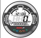
In the fuel, volt screen, hold pressing the Select Button for 3 seconds to switch to the RPM screen.
