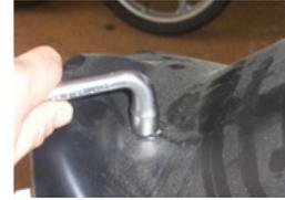
AFTER HAVING WITHDRAWN The DOOR LUGGAGE WITH A TUBULAR HEXAGON BOX SPANNER TUBE OF 13, TO LEAVE The MASK.
