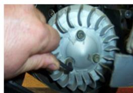
REPOSITION The 3 SCREWS Of ORIGIN OF The SUPPORT OF THE VENTILATOR WITH A ALLEN WRENCH OF 5
