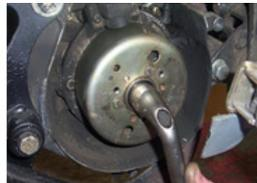
TURN THE ROTOR IN SENS REVERSES OF THE DIRECTION OF ROTATION SO THAT The VIENNA PISTON IN CONTACT WITH The BLOCK PISTON, LOOSEN the NUT OF The ROTOR WITH A TUBULAR HEXAGON BOX SPANNER TUBE OF 16.
