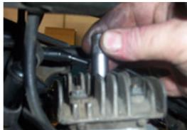
WITHDRAW The CANDLE AND TO PLACE A BLOCK PISTON A ITS SITE
