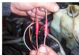
CONNECT THE CABLES OF THE STATOR AND THE DIAGRAM, BLACK/RED UNIT AND WHITE/RED UNIT
