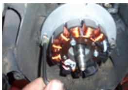
PASS The SHEATH Of IGNITION MILLÉNIUM BY The HOLE OF The CASING OF ORIGIN AND POSITION The TURNTABLE BY PRESENTING A FASTENING SCREW OF ORIGIN ON HOLE REPERE "V" OF The TURNTABLE, PRESENT The SECOND SCREW AND TIGHTEN the WHOLE WITH A ALLEN WRENCH OF 5
