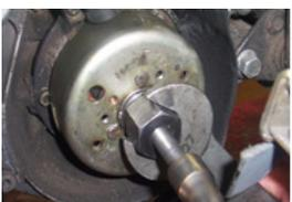
POSITION EXTRACTOR MBK AND YAMAHA. ATTENTION, IT SCREWS A BACK AND TO EXTRACT The ROTOR Using The CORRESPONDING KEYS
