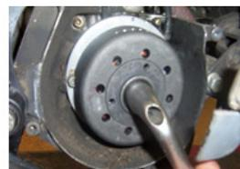
PRESENT the NUT Of ORIGIN AND TO TIGHTEN WITH A TUBULAR HEXAGON BOX SPANNER TUBE OF 16.
