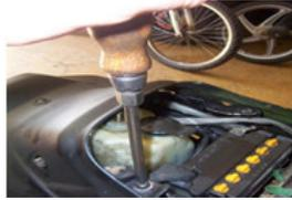
WITHDRAW THE 2 HIGHER SCREWS OF THE MASK BELOW OF SADDLE WITH A PHILLIPS SCREWDRIVER.
