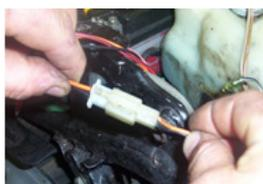
CONNECT THE CONNECTOR 2 WAYS OF THE DIAGRAM WITH THAT OF THE BEAM BLACK CABLE UNIT AND ORANGE CABLE UNIT.
