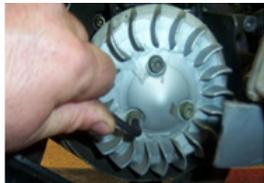
WITHDRAW THE 3 SCREWS SUPPORT OF THE VENTILATOR WITH A ALLEN WRENCH OF 5.
