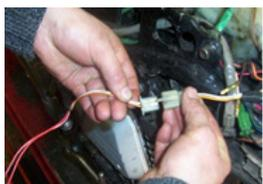
PASS BY AGAIN The SHEATH OF STATOR MILLÉNIUM ALONG The FRAME LIKE ORIGIN AND CLIPSER CONNECTORS 3 WAYS OF The STATOR AND BEAM, YELLOW/RED CABLE UNIT AND WHITE TOGETHER.
