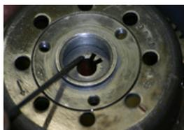
PRESENT The ROTOR ON The VILBREQUIN BY PUTTING GROOVE "A" ON The KEY OF The CRANKSHAFT. W IRING THE FRAME.
