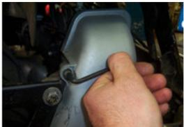
WITHDRAW THE SCREWS SUPPORT OF THE MASK IGNITION WITH A ALLEN WRENCH OF 5 AND WITHDRAW IT.
