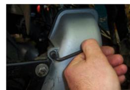
PRESENT THE SCREWS OF THE SUPPORT OF THE MASK IGNITION WITH A ALLEN WRENCH OF 5.
