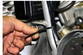
Place the 2 plastic collars on the tube, like at the origin.
