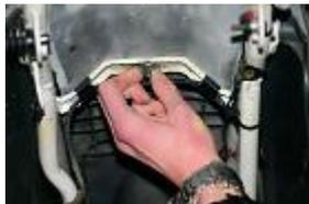
Remove the butterfly nut under the saddle.
