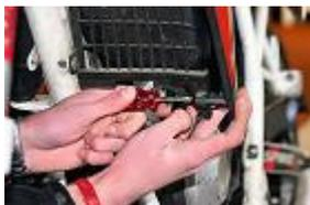
Remove the inferior fixation screws from the left and right side around the radiator.
