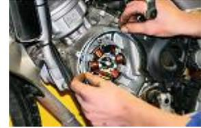
Remove the air tightness joint of the ignition cover.
