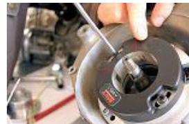
Recover the wire pass of the original stator and place it in the right way on the tube of the PREMIUM stator. Put the PREMIUM stator on the support: put the tube by the carter hole and tighten it with the 2 provided screws of 5x30mm.
