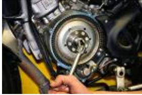
Loosen the nut with a key of 15.
