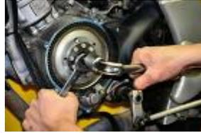
Screw the extractor for the **DUCATI** ignition and remove the rotor with the 2 corresponding keys.
