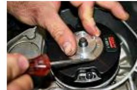
Loosen the block piston stick and use it like a stick, turning the crankshaft to find the BTDC. At the BTDC, make the marks coincide the 2 red marks of the stator and the rotor agree and tighten the rotor with the disc and the original nut.
