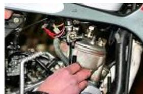
After closing the tap, remove the petrol pipe.
