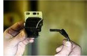
Screw the cable on the high voltage coil and lower protection on the original high voltage coil.
