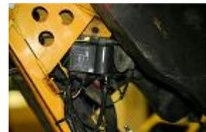
Remove the high voltage coil disconnecting all the cables.
