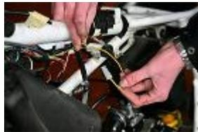
Connect the yellow cable of the stator with the yellow wiring harness.
