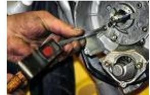
Caution! The 3 screws of the support are very difficult to unscrew! To do this, use an Allen key of 3 and give small blows with a hammer before trying to remove its.
