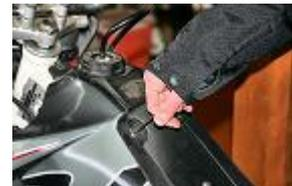
Remove the superior fixation screws, from the right and left sides. on the tank.
