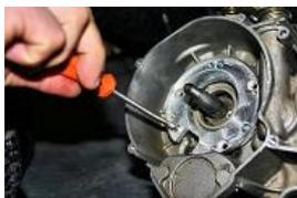
Put the PREMIUM support and to tighten it with the 3 provided screws and with a cross-shaped screwdriver.
