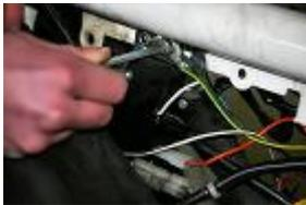
Place the high voltage coil at its original place, with the 2 original screws of 6 mm without forgetting the green/yellow cables of stator, black of the frame and black of the diagram.
