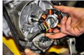
Disconnect the yellow cable and remove the stator and its rubber shutter.
