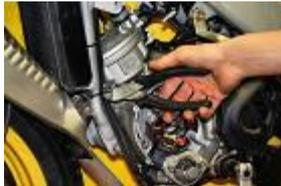
Cut the inferior plastic collar of the sheath until the high voltage coil.
