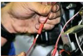
Put together the black/red cable of the diagram and the stator.
