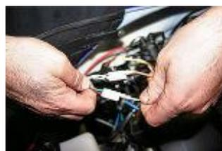
Connect the white/black cable of the MVT diagram on the green cable of the 2 ways connector, previously connected on the original connector.
