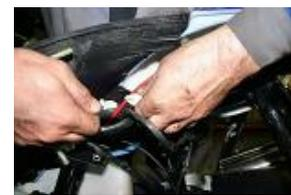
**Disconnect the individual cables and the stator connector.**
