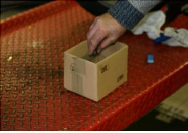
Prepare a pack, before beginning, to tide all the screws removed, in order to find them back for the reassembly.
