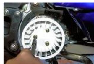
Reassemble the ventilator with the 3 cross-shaped screws.
