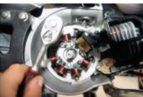
**Remove the stator, with a key of 8 and remove the wiring harness.**
