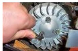
Tighten the ventilator with the training fingers of the water pump, for the liquid models, with the original screws.
