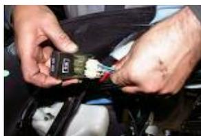
**Remove the original CDI and disconnect the 2 connectors.**
