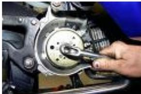
**Loosen the rotor nut, with a key of 17.**
