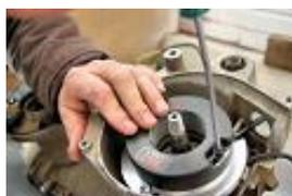
Put the cables stator through the original carter hole and tighten the stator on the support with the 2 provided Allen screws of 5x30 mm.
