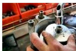
Fit the block piston stick, tightening it slowly and tighten the rotor with the original nut. Then, when the rotor is tightened, check the red marks meet at the BTDC.
