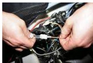
Connect the orange cable of the MVT diagram on the white/black cable of the 4 ways connector, previously connected on the original
