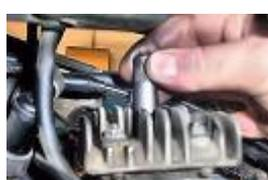
Unscrew the block piston stick and turn the crankshaft to find the BTDC, using the block piston stick.
