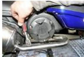
**Remove the screws with a key of 8, and the superior cross-shaped screw, to remove the ignition cover.**
