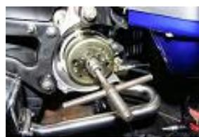
**Place the extractor MBK and YAMAHA and remove the rotor.**
