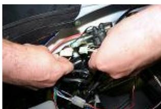
Connect the 3 ways connector of the MVT stator with the 3 ways connector of the wiring harness; and the stator black cable with the MVT diagram black cable.
