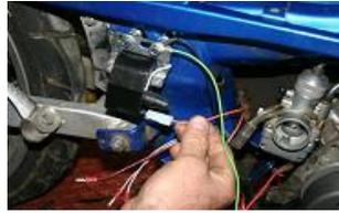
Connect the orange cable of the diagram to the high coil.
