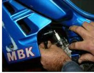
Withdraw the spark plug cap.
