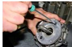
Feat the support with the two screws 6x20 milled heads and control if the support is correctly on the engine without any screws of casing does not obstruct.
