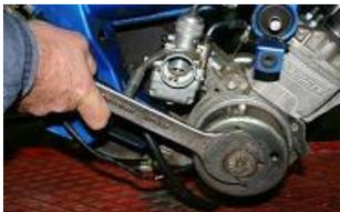
Turn the crankshaft to block the piston on the stick and Loosen the nut with a 32 mm key.
