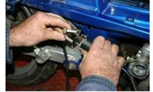
Deposit of the original high voltage coil.
