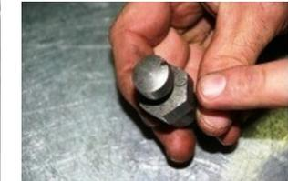
Find a timing stick adjustable Screw the timing stick at the place of the spark plug.
