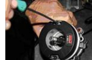
Place the stator DD on the support and screw it with the two allen screws delivered.
