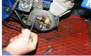
Deposit the fastening screws of the stator.
