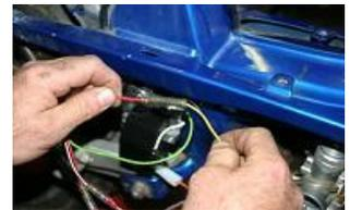
The cables yellow for the regulator bulbs 12 v 5 watts behind and 12v 15 w in front the cables white mustn't be connect. To stop the engine you can also connect the black and white cables to a switch connect to the mass (metal body of the engine).
