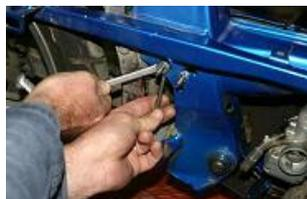
Place the 6x 35mm screws delivered with the plates and nut of 6 MM To fit the MVT high voltage coil.
