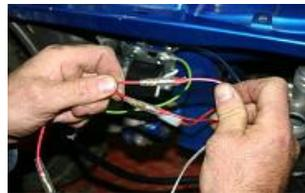
The cables black red of the diagram with the same colour on the stator.
