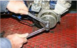
With the extractor MBK withdraw the rotor of the original ignition.
