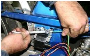
Joint the green cable of the stator with the black cable of the Diagram to the metal body of the MVT high voltage coil.
