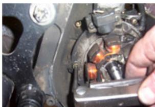
DEPOSIT THE STATOR WITH A ALLEN KEY OF 5 AND TO WITHDRAW THE BEAM OF THE FRAME, BUT KEEP THE PAPER SEAL.
