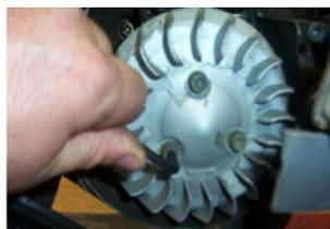
REMOVE THE 3 SCREWS SUPPORT OF THE VENTILATOR WITH A ALLEN KEY OF 5 AND DEPOSIT IT.
