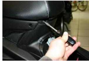
REMOVE THE 2 SCREWS OF THE FRONT PLASTIC PROTECTION UNDER THE SADDLE.
