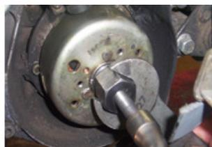
REMOVE THE MECAN NUT OF The ROTOR WITH HELP OF YAMAHA EXTRACTOR. CAUTION THREAD IS REVERSE.
