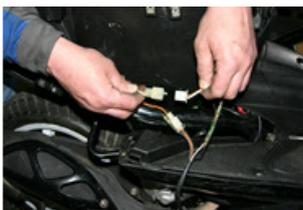
DISCONNECT THE 3 WAYS CONNECTOR FROM THE STATOR AND REMOVE PLASTIC COLLAR ON THE CABLE OF THE STATOR.
