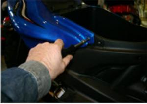
OPEN THE SADDLE AND REMOVE THE FRONT SCREW OF THE RIGHT BACK PLASTIC PROTECTION.
