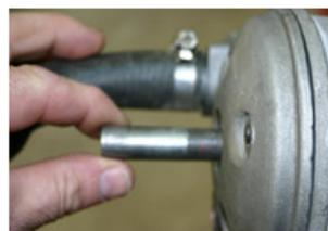
IF YOU DO NOT HAVE A AIR GUN, WITHDRAW The SPARK PLUG AND TO INSTALL A STICK.
