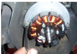
PASS THE BLACK CABLE INSIDE THE CASE EXIT HOLE AND PUT A ORIGINAL SCREW ON THE HOLE H OF THE STATOR, PLACE THE SUPPORT ON CASE AND SCREW IT. PASS THE BLACK CABLE INTO THE ORIGINAL HOLE CASE AND CLOSE THE WINDOW WITH THE LATEX OPTURATOR.
