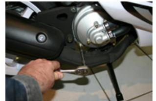
REMOVE THE WATER PUMP WITH ALLEN KEY OF 5 mm
