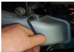
FOR AIR COOLED MODEL, REMOVE THE PLASTIC COVER OF THE IGNITION.
