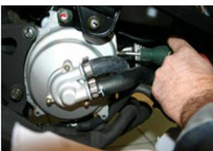
WITHDRAW THE 2 FASTENING SCREWS OF THE MASK FRONT IGNITION WITH A MINI PHILLIPS SCREWDRIVER WHILE DRAWING ON BOTTOM FROM CASE TO HAVE ACCESS
