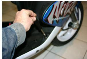
REMOVE THE FRONT SCREW OF THE FEET SUPPORT.
