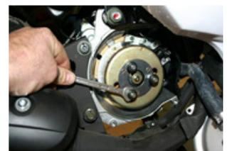
TURN ROTOR WITH HAND TO COME TO PUT The PISTON IN CONTACT WITH THE STICK, DISMOUNT The 3 PINS OF PUMP WATER WITH A 10 mm KEY.
