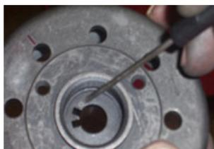
PRESENT The ROTOR WITH THE KEY CRANKSHAFT ON THE GROOVE A.
