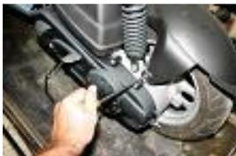
Remove the left screw from the back mudguard.
