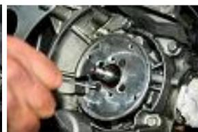
Drill the 2 carter thread on 1 mm and check the thread.
