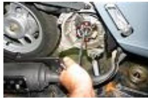
Remove the 2 fixation screws from the stator.
