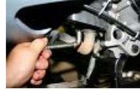
Remove the 2 fixation nuts of the exhaust with a key of 10.
