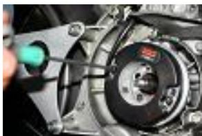
Put the Premium cables through the hole in the carter and tighten with 2 provided screws of 5x25mm.
