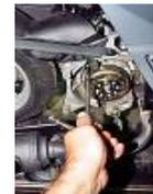
Remove the pick up from the original ignition.
