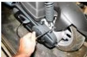
Reassemble the back mud-guard like at the disassembly.
