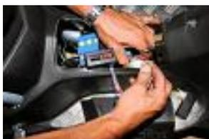
Put the RJ051X MVT diagram at the original CDI place. For the models with a Dellorto ACPH1 CDI, use a RJ054X diagram, put the red clip on the black cable of the CDI without disconnecting it. Put the brown cable not bared in parallel of the black on the clip and close the clip with pliers in order the 2 cables are joined in parallel without cutting the black cable of the diagram.
