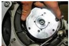
Put the PREMIUM rotor on the crankshaft, placing the two red marks of rotor and stator, at BTDC.
