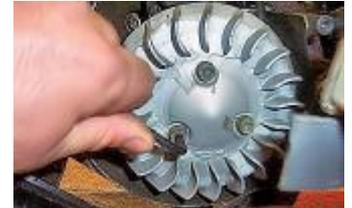
Remove the 3 support screws of the ventilator with an Allen key of 5.
