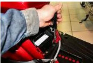
Remove the 2 front screws of the under saddle with a cross-shaped screwdriver.
