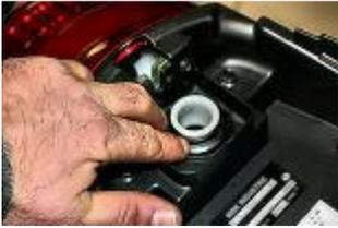
Remove the air tightness seal between the oil tank and the back. And remove the back, slowly pulling on the saddle.
