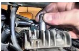
Remove the block piston stick and place the spark plug with its connector cap.
