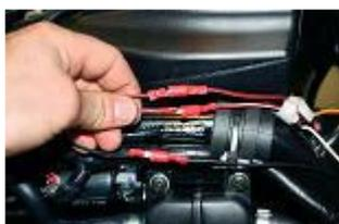
Connect the red/black cables of the diagram and of the stator, together.
