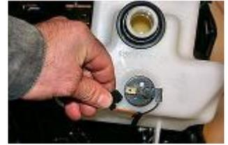
Remove the 2 cables of the level sounding of the expansion tank.
