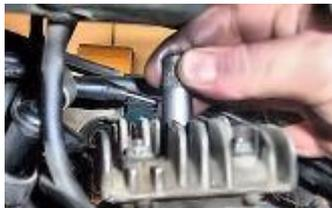
Remove the spark plug and place a block piston stick at its place.
