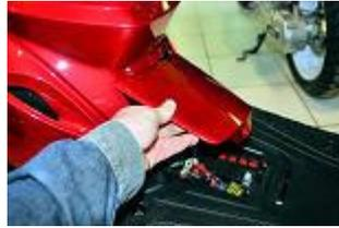
Remove the battery cover with a cross-shaped screwdriver.
