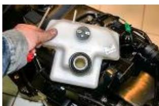
Replace the expansion tank for the BOOSTER ROAD model.
