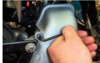
Remove the support screws of the ignition cover with an Allen key of 5 and remove it.
