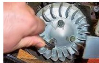
Tighten the ventilator or the training fingers of the water pump for the liquid models with the original screws.
