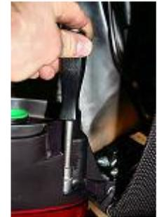
Remove the 2 right and left screws of the back with a key of 10.
