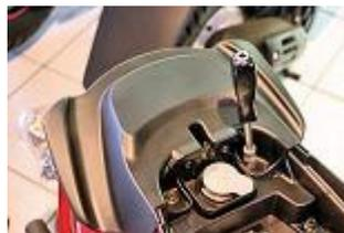
Remove the 2 back screws of the spoiler with a key of 10.
