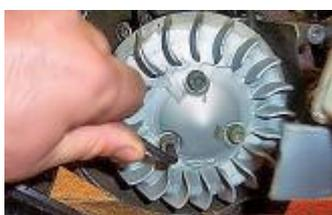
Place the 3 original screws of the ventilator support with an Allen key of 5.
