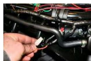
Remove the orange cable of the original high voltage coil.
