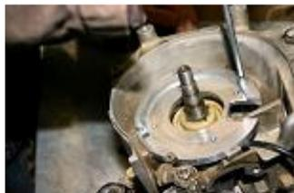
Place the support keeping the paper seal and tighten it with 2 original Allen screws of 6.
