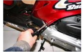
Remove the front left screw from the under saddle cover.
