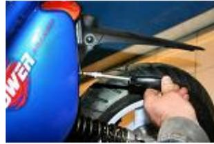
Remove the central fixation screw of the left under saddle.
