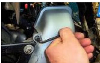
Reassemble the carter protection with the original screws.
