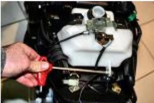
Remove the support screw of the expansion tank with an Allen key of 5.
