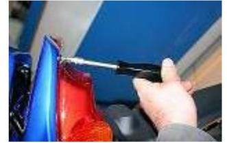
Remove the back fixation screw of the left under saddle cover.
