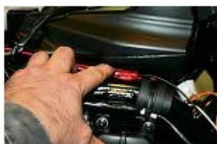
Place the cables under the plastic cover of the under saddle to protect it.
