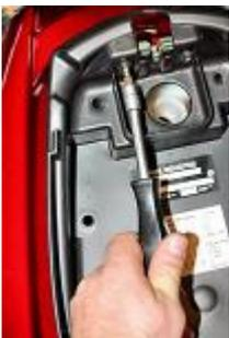
Remove the blockade of the seat and set with a star screwdriver.
