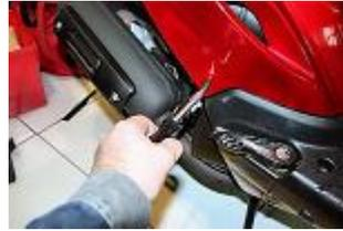
Remove the front right screw from the over saddle cover.
