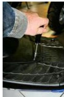
Remove the fixation screws of the front under saddle cover with a cross-shaped screwdriver.
