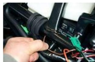
Put the brown cable below the frame tube to the original CDI.
