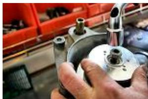
Fit the block piston stick: Tighten the block piston stick and tighten the rotor with its original nut. After have tightned the rotor, check the 2 red marks coincide to the BTDC.
