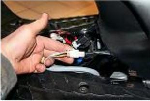
Disconnect the connector joining the stator to the cables located over the battery and cut the plastic collar holding the sheath of the stator along the frame, until the engine carter.
