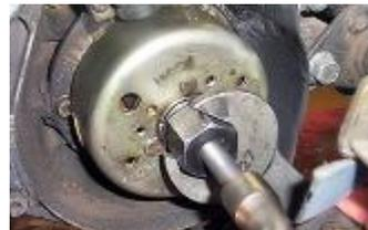
Place the extractor MBK or Yamaha. Remove the rotor with the corresponding keys.
