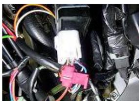
Put the red provided clip on the brown cable of the original CDI and place the brown cable of the diagram in the second place of the clip and close it with a clip in order to put in touch the 2 brown cables.
