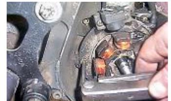
Remove the 2 support screws of the stator with an Allen key of 5, and remove the stator from the carter.
