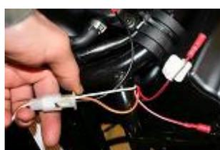
After place the stator Premium tube along the frame and set it with plastic collar, connect the 4 ways connector of the stator with the one of the wiring harness.
