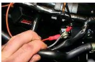
Connect the orange cable of diagram on the high voltage coil. And after have loosened one of the coil fixation screws, screw the black cable of the earth diagram.
