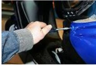
Remove the front fixation screw of the under saddle cover.
