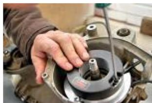
Put the cables of the stator through the original hole of the carter and tighten the stator on the support with 2 Allen provided screws of 5x30mm.
