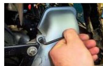
Reassemble all the support screws of the ignition cover with an Allen key of 5.
