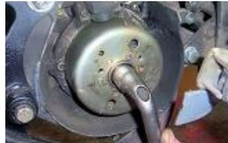
Turn the rotor in the opposite way of rotation in order to put in touch the piston with the block piston stick. Loosen the rotor nut with a key of 16.
