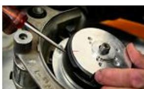
Place the rotor on the crankshaft placing the red marks of stator and rotor the one in front the other.
