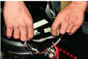
Disconnect the connector joining the stator to the wiring harness which is located over the battery and cut the plastic collar holding the stator tube along the frame until the engine carter.
