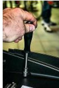
Remove the 2 front screws of the spoiler with a key of 10.
