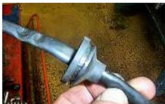
Recover the wire pass of the original stator tube, in order to place it on the Premium tube.
