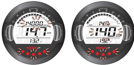
$\geq$  Maximum display value 14,000 RPM
