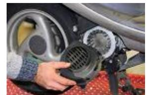
**REMONTER LE CACHE ALLUMAGE AVEC DES VIS DE 5 MM PLUS LONGUE ET 3 ENTRETOISES DE 7 MM. POUR LES MODELS AIR POSITIONNER 1 BANDE SCOTCH AMERICAIN NOIR POUR ASSURER L'ETANCHEITE.**
