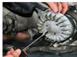
**RETIRER LA VENTILETTE DU ROTOR D'ORIGINE.**
