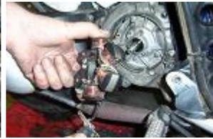
**DEPOSER LE STATOR EN RETIRANT SA GAINÉ D'ALIMENTATION ET SON PASSE FIL.**
