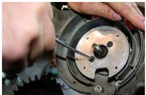
**MONTAGE DE LA ROTOR PLATINE A L'AIDE DE 2 VIS 5 X 16 TETE FRAISEE FOURNIES ET CONTROLER LE CALAGE AU**
