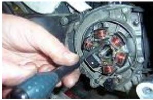
**RETIRER LES VIS DE FIXATION DU STATOR AVEC UN TOURNEVIS CRUCIFORME.**
