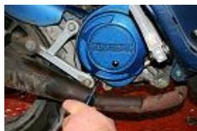
POUR LES MODELES DES LIQUIDES, RÉ FIXER LE CACHE D'ALLUMAGE D AVEC DES VIS PLUS LONGUE ET 3 ENTRETOISES DE 7 MM.
