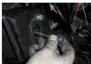
**SI VOUS NE POSSEDEZ PAS LE PISTOLET A AIR COMPRIME, RETIRER LA BOUGIE ET PLACER UN BLOQUE PISTON A SON EMPLACEMENT.**
