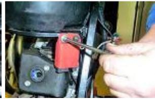
**DEPOSER LES DEUS VIS DE FIXATION DE LA BOBINE HAUTE TENSION AVEC UNE CLE A PIPE DE 8 ET LA RETIRER.**
