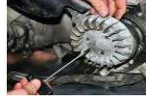
POUR LES MODELES A AIR, REPOSITIONNER LA VENTILETTE D'ORIGINE AVEC LES 3 VIS DE 5 X 12
