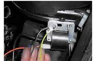
**PLACER LA BOBINE A L'EMPLACEMENT D'ORIGINE ET SERRER AVEC**
