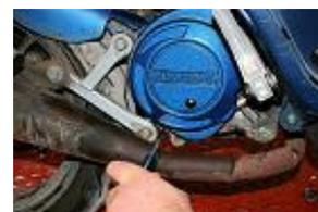
**POUR LES MODELES A REFROIDISSEMENT LIQUIDE, RETIRER LES VIS DU CACHE ALLUMAGE AVEC UN TOURNEVIS CRUCIFORME.**
