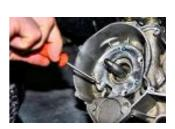
PRESENTER LA PLATINE PREMIUM ET LA SERRER AVEC LES 3 VIS FOURNIES A L'AIDE D'UN TOURNEVIS CRUCIFORME.
