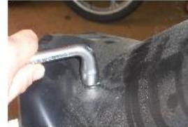
APRES AVOIR RETIRE LE PORTE BAGAGE AVEC UNE CLÉ A PIPE DE 13, SORTIR LE CACHE.
