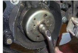
TOURNER LE ROTOR DANS LE SENS INVERSE DU SENS DE ROTATION POUR QUE LE PISTON VIENNE EN CONTACT AVEC LE BLOC PISTON, DESSERRER L'ÉCROU DU ROTOR AVEC UNE CLÉ A PIPE DE 16.
