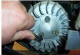
RETIRER LES 3 VIS SUPPORT DE VENTILLETTE AVEC UNE CLÉ ALLEN DE 5.
