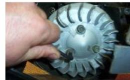
REPOSITIONNER LES 3 VIS D'ORIGINE DU SUPPORT DE VENTILLETTE AVEC UNE CLÉ ALLEN DE 5.
