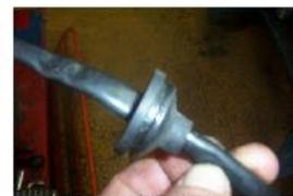
RÉCUPERER LE PASSE FIL SUR LA GAINÉ DU STATOR D'ORIGINE POUR LA PLACER SUR LA GAINÉ DU MILLÉNIUM.
