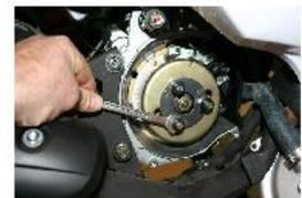
TOURNER LE ROTOR A LA MAIN POUR VENIR METTRE LE PISTON EN CONTACT AVEC SON BLOCAGE, DÉMONTER LES 3 ERGOTS DE POMPE A EAU AVEC UNE CLÉ PLATE DE 10.
