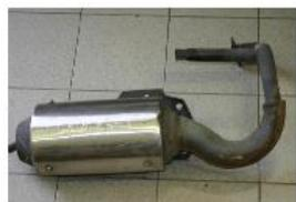
DÉPOSE DU POT D'ÉCHAPEMENT.
