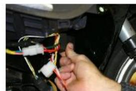
REPOSITIONNER LE DIAGRAMME AVEC SON SUPPORT CAOUTCHOUC A L'EMPLACEMENT D'ORIGINE.
