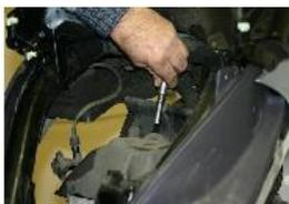
DÉMONTÉ LE BLOQUE PISTON, REPOSITIONNER LA BOUGIE ET SON ANTI PARASITE.
