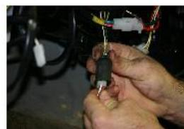
REPOSITIONNER LA PROTECTION ANTI HUMIDITÉE SUR LE CONNECTEUR DU DIAGRAMME.
