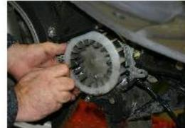
EN UTILISANT UNE CLÉ A PIPE DE 8, REMONTER LA TURBINE A L'AIDE DES 4 VIS DE 5 mm D'ORIGINE.
