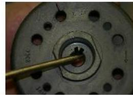
PRÉSENTER LE ROTOR SUR LE VILBREQUIN EN PLACANT LA CLAVETTE SUR LA RAINURE "A" COMME ANALOGIQUE (VOIR PHOTO CI-DESSUS).
