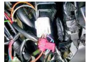
**POSITIONNER LE CLIP ROUGE FOURNI SUR LE CABLE MARRON OU CABLE ROUGE / BLANC POUR LES MODELS A PARTIR DE 2008 DU CDI D'ORIGINE SANS LE DECONNECTER NI LE COUPER, PLACER LE CABLE MARRON DU DIAGRAMME EN PARALLELE SUR LE CLIP A COTE DU CABLE MARRON DU CDI ET FERMER LE CLIP AVEC UNE PINCE POUR QUE LES 2 CABLES SE METTENT EN CONTACT.**
