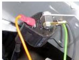
**RETIRER LE CABLE ORANGE DE LA BOBINE POUR LE REMPLACER PAR LE CABLE ORANGE DU DIAGRAMME. RETIRER LA VIS SUPPORT DE LA BOBINE HAUTE TENSION ET RE FIXER EN CONSERVANT LE CABLE NOIR D'ORIGINE AINSI QUE LE CABLE NOIR DU DIAGRAMME ET VERT / JAUNE DU STATOR.**
