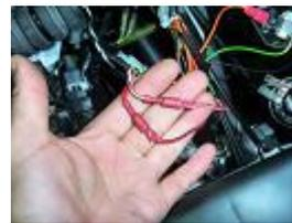
**CONNECTER LES CABLES NOIR / ROUGE DU DIAGRAMME ET DU STATOR ENSEMBLE.**
