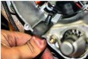
**PLACER L'OBTURATEUR DE FAÇON A FERMER LA SORTIE DE CABLE DU CARTER.**
