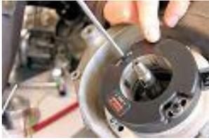
**RECUPERER LE PASSE FIL DU STATOR D'ORIGINE ET LE POSITIONNER DANS BON SENS SUR LA GAINÉ DU STATOR PREMIUM. PRESENTER LE STATOR PREMIUM SUR LA PLATINE EN PASSANT LA GAINÉ PAR LE TROU DU CARTER ET LE SERRER AVEC LES 2 VIS 5 X 30 MM FOURNIE.**
