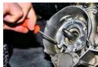
**PRESENTER LA PLATINE PREMIUM ET LA SERRER AVEC LES 3 VIS FOURNIES A L'AIDE D'UN TOURNEVIS CRUCIFORME.**
