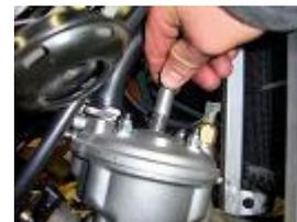
**METTE A LA PLACE DE LA BOUGIE UN BLOC PISTON ET TOURNER A LA MAIN LE ROTOR POUR METTRE LE PISTON EN CONTACTE AVEC SON BLOCAGE.**
