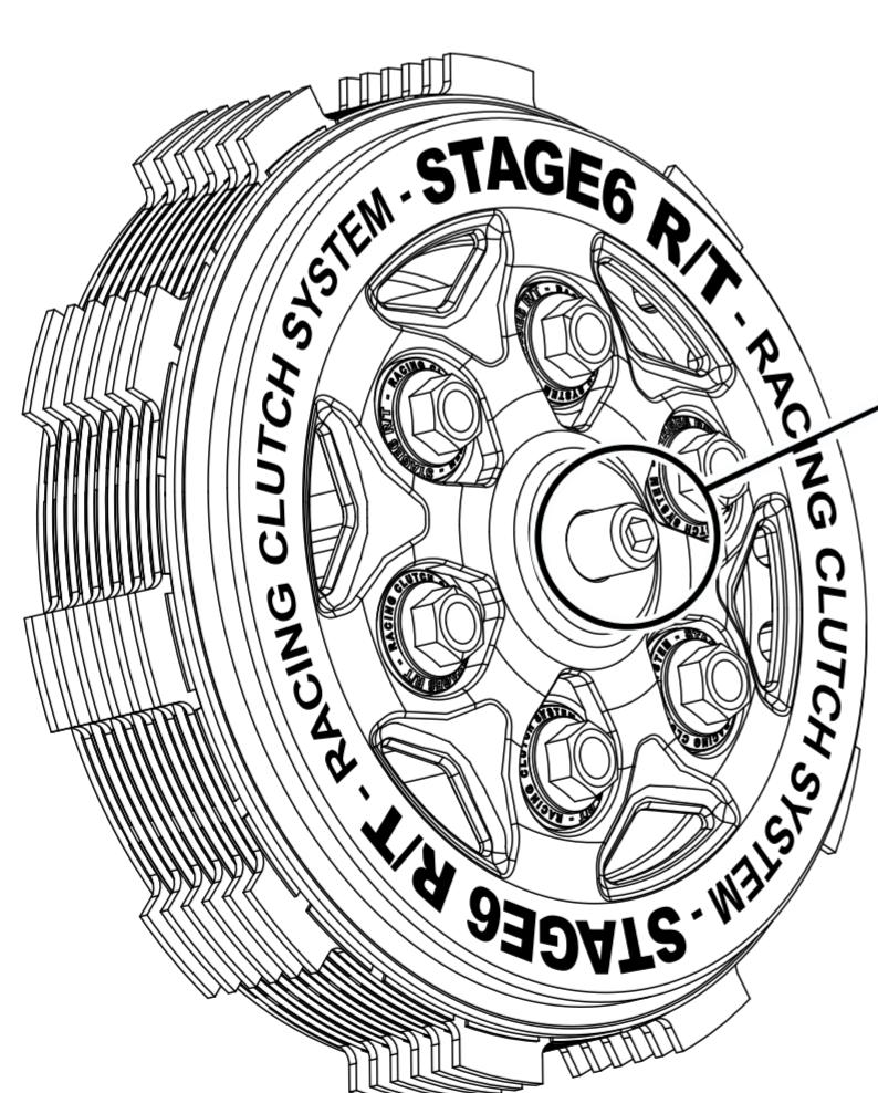
SCREW THE CLUTCH PUSH ROD
