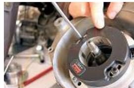
Recover the wire pass of the original stator and place it in the right way on the tube of the DIGITAL DIRECT stator. Put the DIGITAL DIRECT stator on the support: put the tube by the carter hole and tighten it with the 2 provided screws of 5x30mm.
