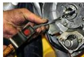
Caution! The 3 screws of the support are very difficult to unscrew! To do this, use an Allen key of 3 and give small blows with a hammer before trying to remove its.
