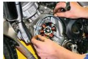
Remove the air tightness joint of the ignition cover.
