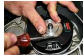
1\_Turn the crankshaft in the rotation side of the engine to block the piston on the stick And find the btdc
