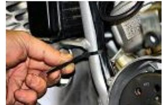
Place the 2 plastic collars on the tube, like at the origin.
