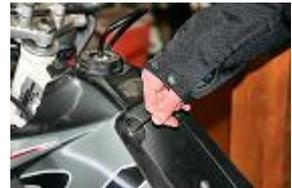
Remove the butterfly nut under the saddle.
