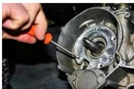
Put the DIGITAL DIRECT support and to tighten it with the 3 provided screws and with a cross-shaped screwdriver.
