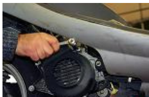
With the key of 8 mm remove the screws from the cover of the ignition.
