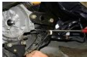
Take out the wiring harness stator opening the clip white wire pass.
