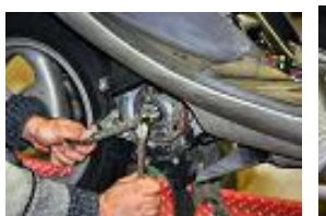
Loosen the nut of 14 which tightens the rotor and screw the Peugeot extractor to remove the rotor, with the corresponding keys.
