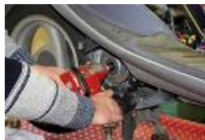
Loosen the nut of 14 which tightens the rotor with a compressed air gun.
