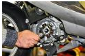
Disassemble the stator with a key of 8.
