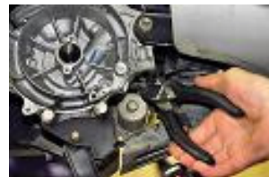
Remove disc holding the exit cable of the ignition and undo above the starter to be able to remove the wiring harness.
