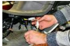
Disconnect the white connector 3 ways and disconnect the black/red cable.
