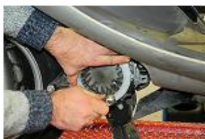
Still with the key of 8 mm, loosen and remove the fixation screws of the ventilator.
