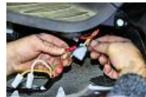
Put the wiring harness stator PREMIUM by the same clips and connect the cables black/red together.
