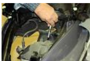
Place a block piston stick at the spark plug place and push slowly down on the kick; turning crankshaft in order to put the piston in touch, with the block piston stick.
