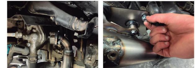
4- Hold the exhaust pipe with one hand while tightening the M6 nuts on the manifold, then tighten the exhaust nuts to the bracket, and finally tighten the bracket bolts to the frame.
