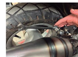
5- Place the inlet nozzle on the muffler with the slot for the spring facing the same direction as the muffler outlet and tighten the 2 M6 nuts on the studs. Insert O-rings into the nozzle channels.
